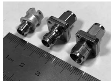
Fig. 5. High-frequency coaxial-to-microstrip and coaxial transitions.
