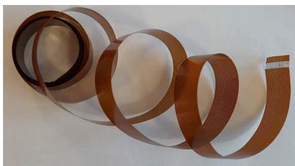
Figure 1. Photograph of a flexible printed cable (FPC).
