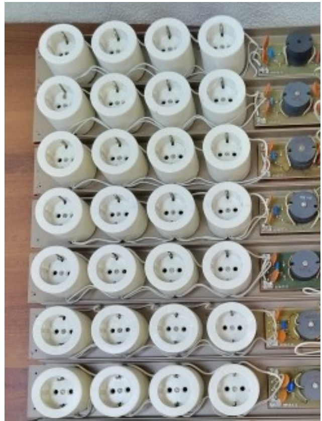
Fig. 2. 10 samples of EMI filters without shielding cases.
