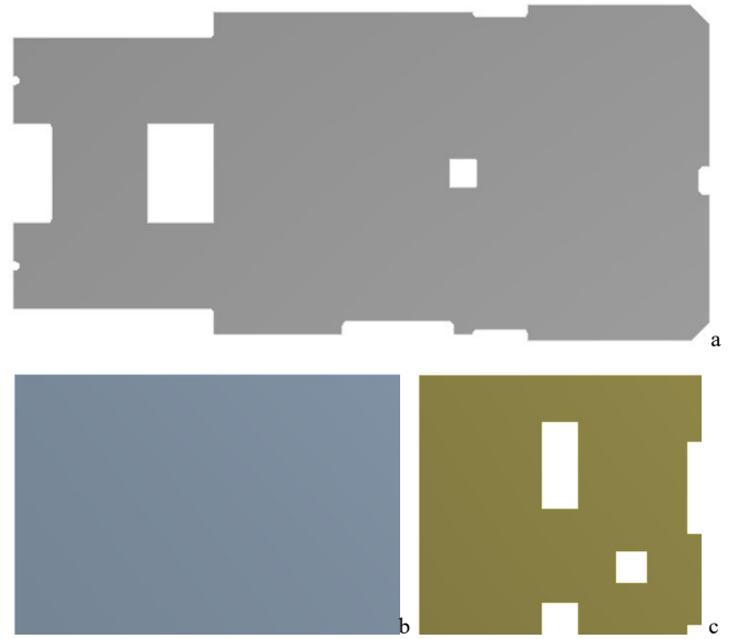
Fig. 5. Simplified models for PCBs of (a) a measuring module, (b) a receiving module, and (c) secondary power sources.
