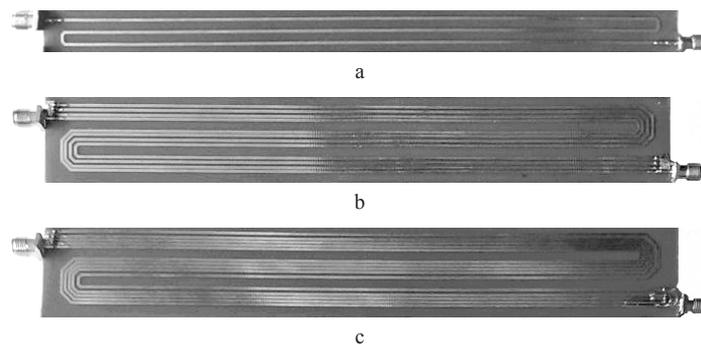
Fig. 2. Prototypes of one- (a), four- (b) and five-conductor (c) MSL
