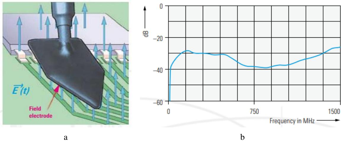
**Figure 4.** Principle of operation (a) and frequency characteristic (b) of the probe RS E 02
