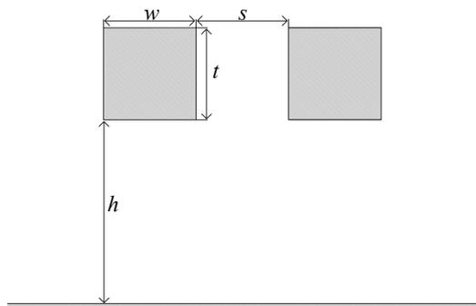
Fig. 1. Cross section of a meander line turn with edge coupling in air filling
