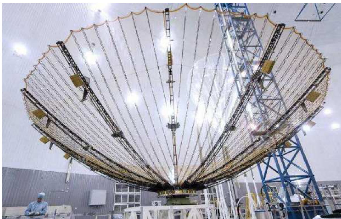
Figure 4. Example of an antenna in the form of a grid of wires as a transformable antenna with gilded wire mesh (mounted on Luch 5A, Luch 5B, and Luch 5V) [259].
