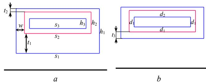
Fig. 3. Cross-sections of the power supply bus in its big (*a*), and small (*b*) parts
