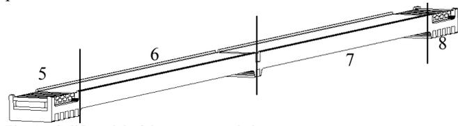
Fig. 1. Solid model of the power supply bus
