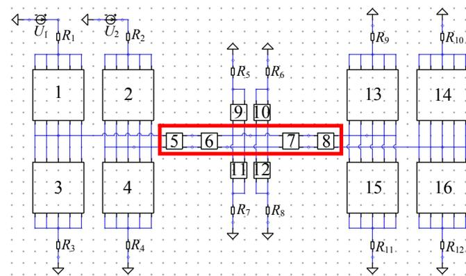
Fig. 2. Circuit diagram of the power supply bus and branch conductors
