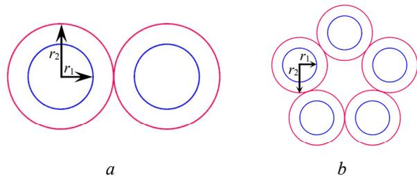
Fig. 4. Cross-sections of the central (*a*), and of the ends (*b*) branch conductors
